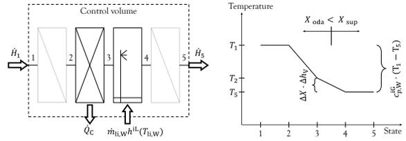
Figure 7 Humidification plus cooling
