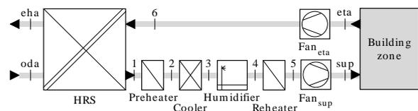
Figure 1 Schematic of an AHU according to (DIN V 18599-3, 2011)
