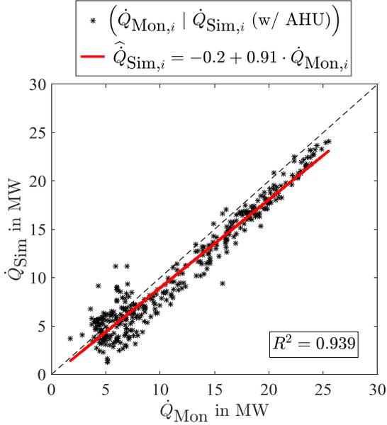
Figure 12 Linear regression analysis of the district simulation
