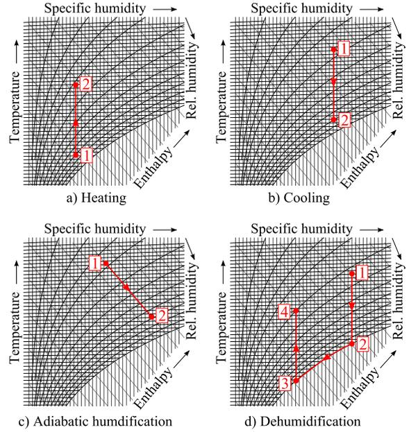
Figure 2 Change of states of moist air in qualitative  $h$ - $X$ -diagrams
