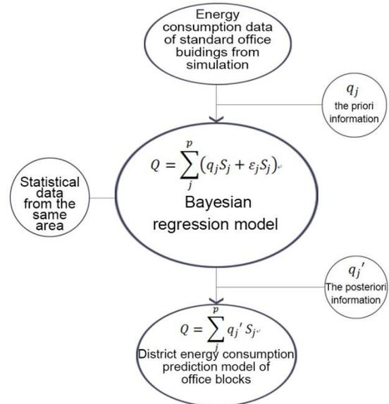
Figure 3 Framework of building the district energy consumption prediction model of office building
