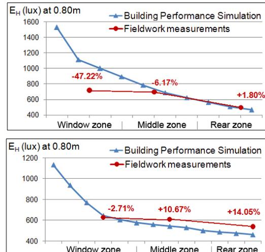
Figure 5 Comparison between BPS and site measurements. Rooms 3.1 (above) and 3.2 (below)
