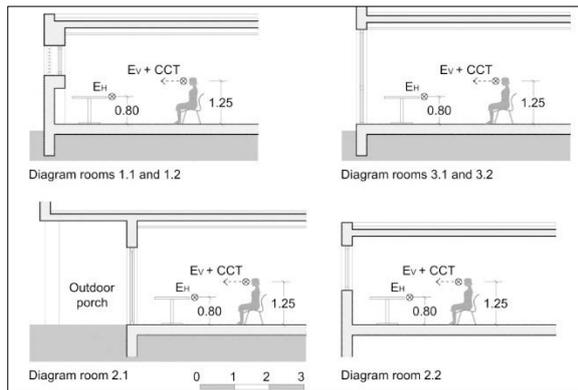
Figure 1 Measurement heights and gaze direction
