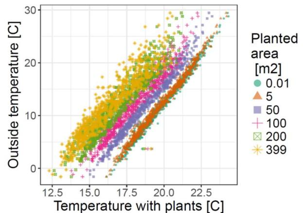
Figure 6: Temperature modelled with the plant module and TRNSYS, as a function of outside temperature, for different planted areas (m<sup>2</sup>).
