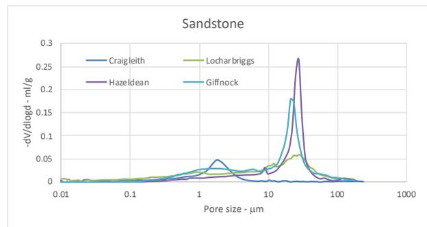
Figure 5: Pore size distributions of sandstones.
