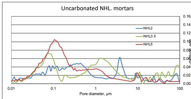
Figure 2: Pore size distributions of uncarbonated NHL mortars.
