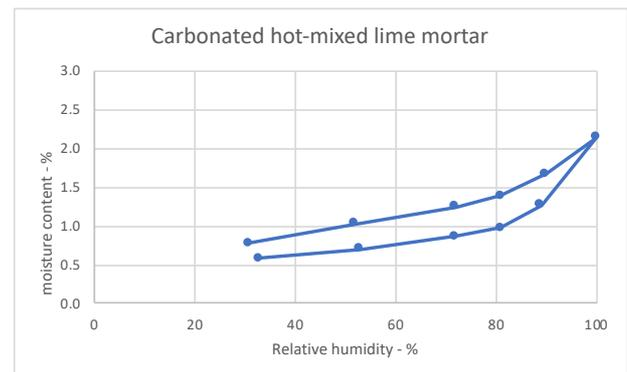
Figure 1: Sorption-desorption curves for carbonated hot-mix lime mortar.
