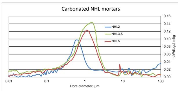
Figure 3: Pore size distributions of carbonated NHL mortars.
