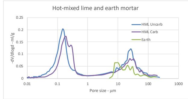
Figure 4: Pore size distributions of hot-mixed lime and earth mortars.
