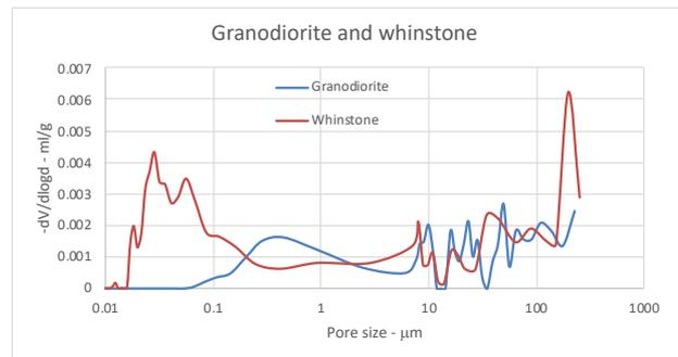
Figure 6: Pore size distributions of granodiorite and whinstone.
