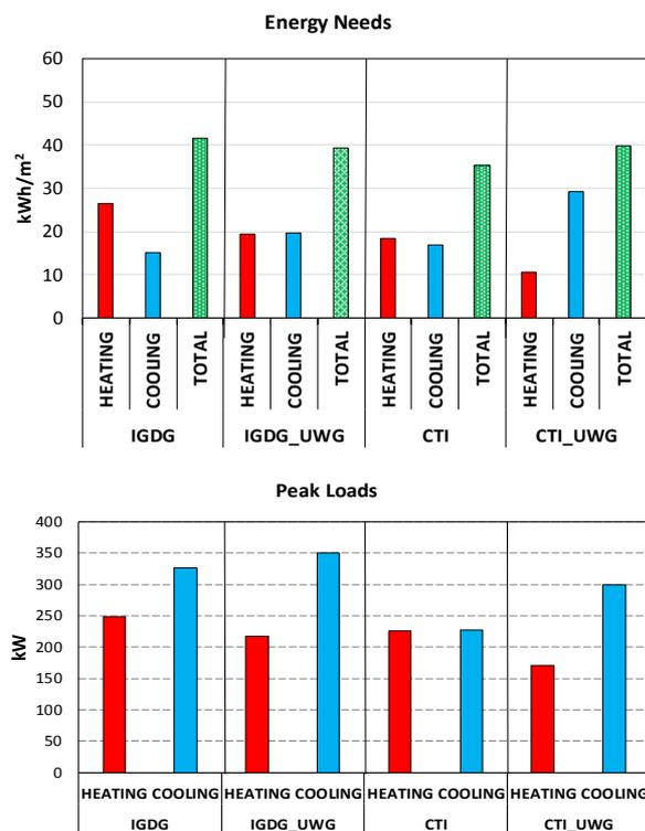
Figure 5: Energy needs (on the top) and peak loads (on the bottom) calculated with the different weather datasets (Insulated envelope scenario)
