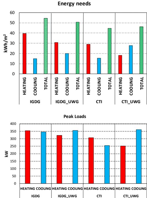
Figure 4: Energy needs (on the top) and peak loads (on the bottom) calculated with the different weather datasets (Uninsulated envelope scenario)
