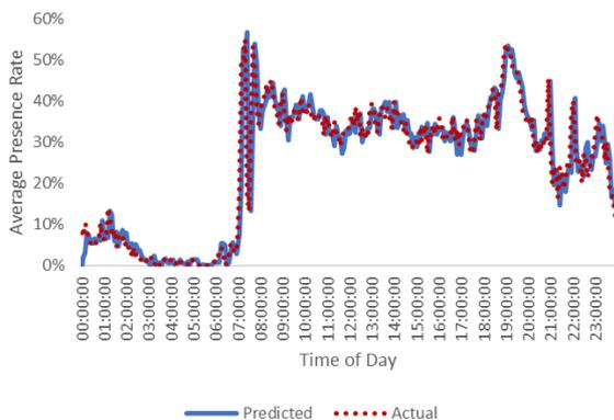
Figure 3: Calibration of the model (building 1)
