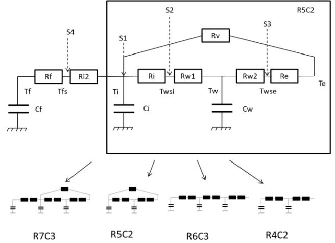
Figure 1: Schematics of the model R7C3 and its derivatives
