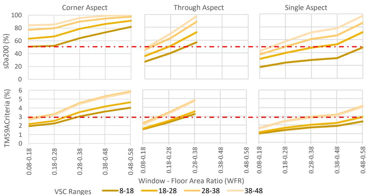
Figure 12: VSC and WFR impact on daylighting and overheating. Red line shows criteria threshold.
