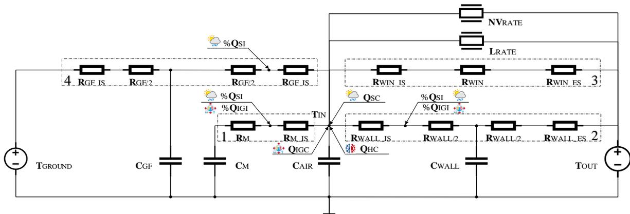
Figure 2 – ROM resistances and capacitance network diagram
