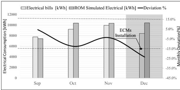
Figure 6 - Comparison of the electrical bills and the ROM electrical energy consumption with monthly deviation for the year 2018
