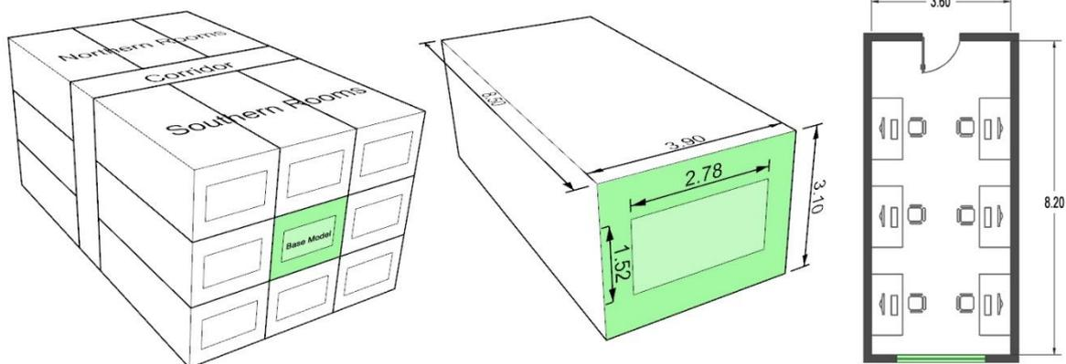
Figure 2- External dimensions of the base model and multiple rooms stacked together to form the building facade. The unit is the meter.
