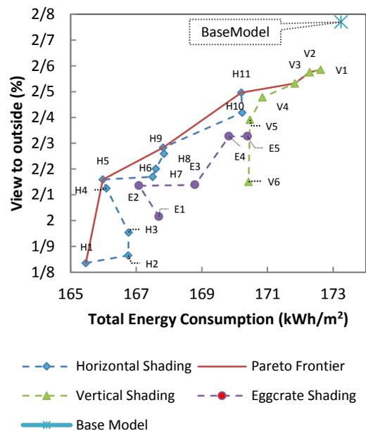
Figure 7- Total optimized shading simulation result
