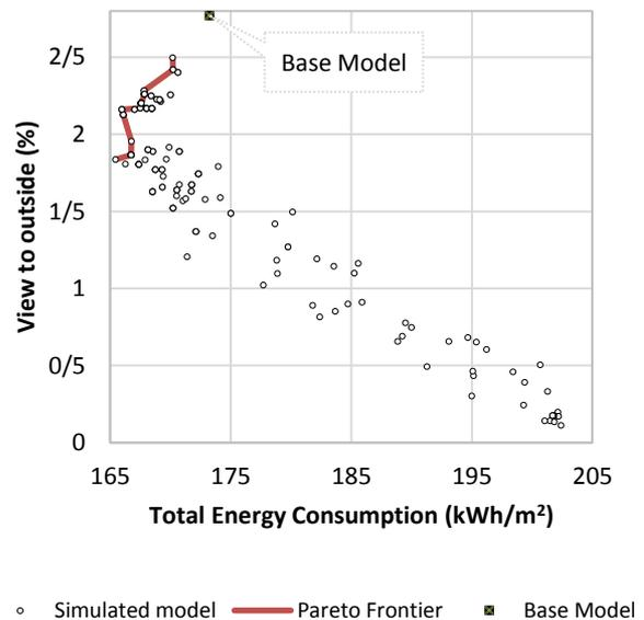
Figure 4- Horizontal shading simulation result.
