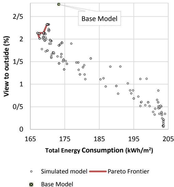
Figure 6- Egg-crate shading simulation result
