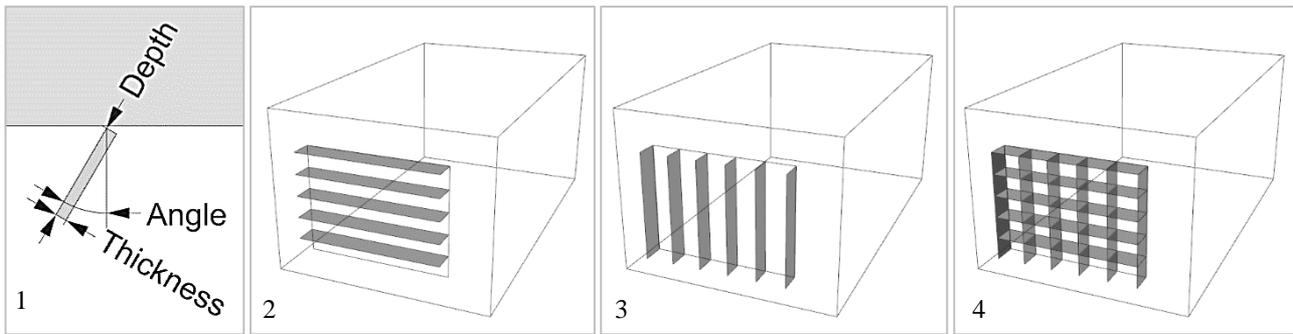
Figure 3- Shading devices. 1: Shading parameters, 2: Horizontal shading, 3: Vertical shading, 4: Egg-crate shading.
