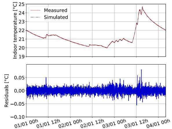
Figure 10: Temperature measured the test cell and estimated by the model and the residuals
