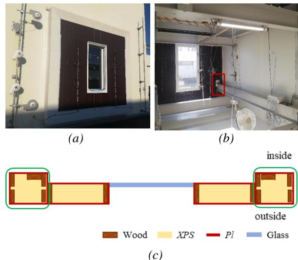
Figure 2: Outside (a) and inside (b) of the test cell (c) Layout of the facade – top view
