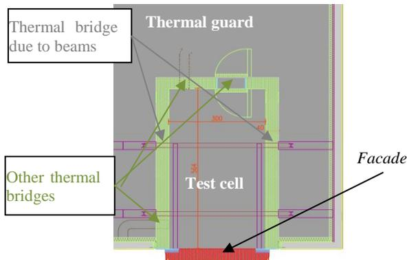
Figure 1: Layout of the facility – top view
