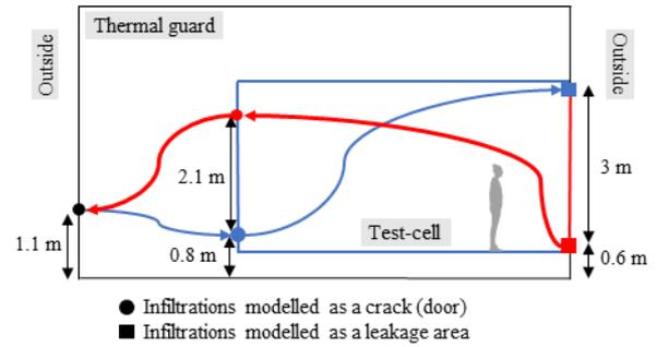
Figure 7: Position of the infiltration openings in the test cell – sectional view
