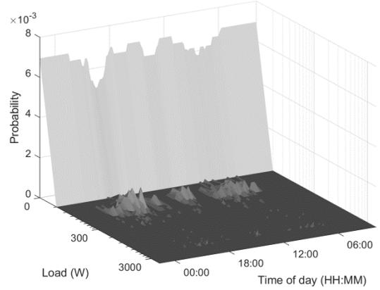
Figure 2: Example distribution of the load measurements for a single washing machine recorded over 18 weekdays, with respect to time-of-day, represented as a histogram.
