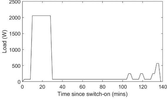
Figure 1: Typical washing machine SULP (Richardson et al., 2010) used in all three models, represented by  $c$
