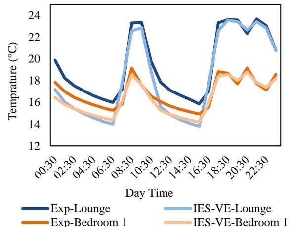
Figure 3. Temperature profile from experiment and IES-VE simulation.
