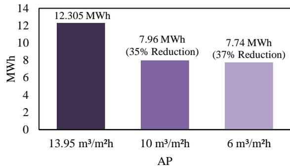
Figure 4. Annual heating energy use pre and post IWI in SEH case study (base line wall U-value of 1.56 W/m<sup>2</sup>K).
