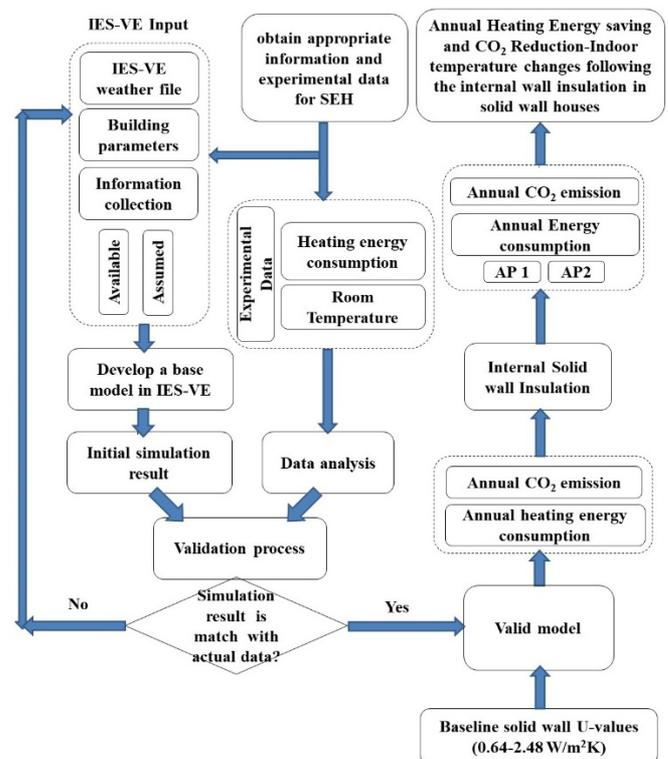
Figure 1. Schematic diagram of the research methodology.
