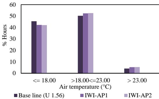
Figure 5. Annual effect of insulation on indoor temperature for SEH (base line U-Value=1.56 W/m<sup>2</sup>K).
