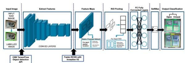
Figure 3: Image of the configured deep learning model for window detection.
