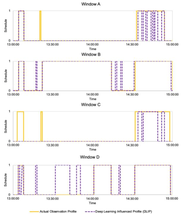
Figure 7: Generated deep Learning Influenced Profile (DLIP) results for window A, B, C, D with corresponding actual observation.
