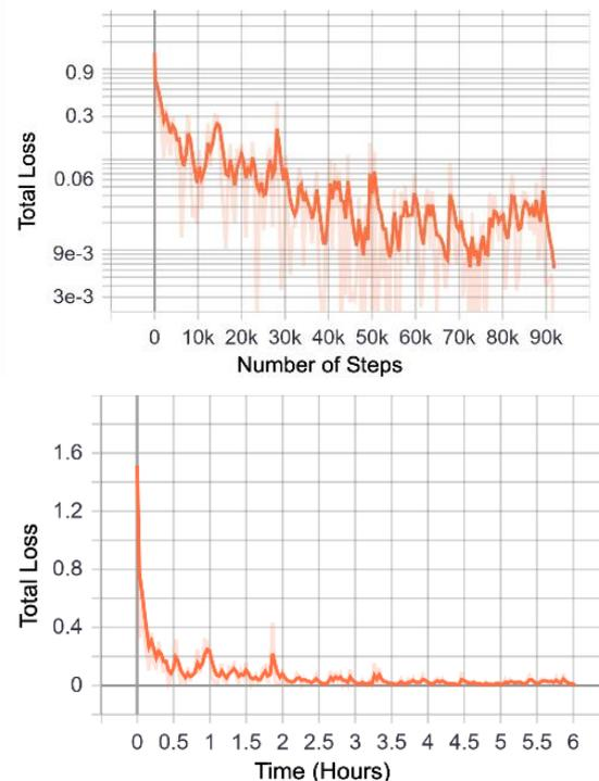
Figure 5: Deep learning model training results using the Faster-RCNN with InceptionV2 model. Total loss against number of a). steps and b). the training time (hours).
