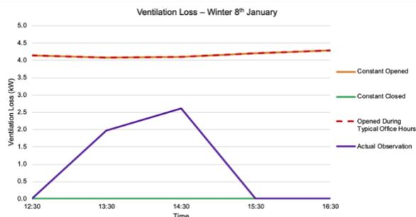
Figure 9: Ventilation loss results for a winter day (8th January) within the two-hour test duration in the lecture room.
