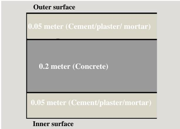
Figure 4: Exterior wall arrangement before applying insulation
