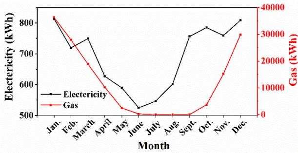
Figure 8: Fuel usage breakdown of RB; Electricity (black curve) and gas (red curve)
