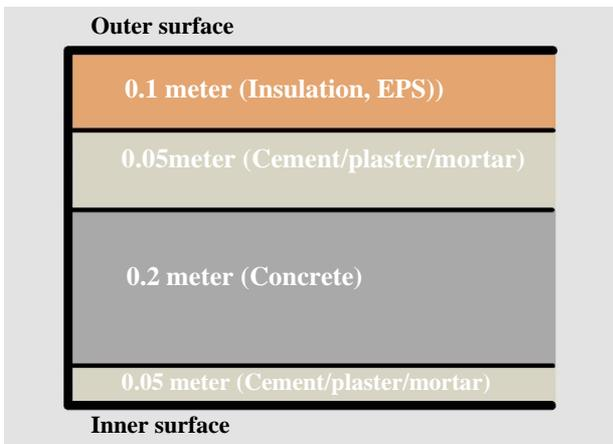
Figure 5: Exterior wall arrangement after applying insulation
