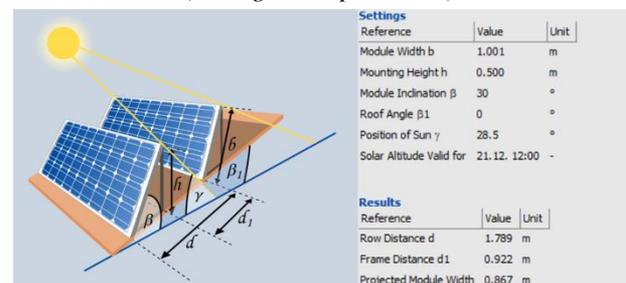
Figure 7: Photovoltaic panels parameters
