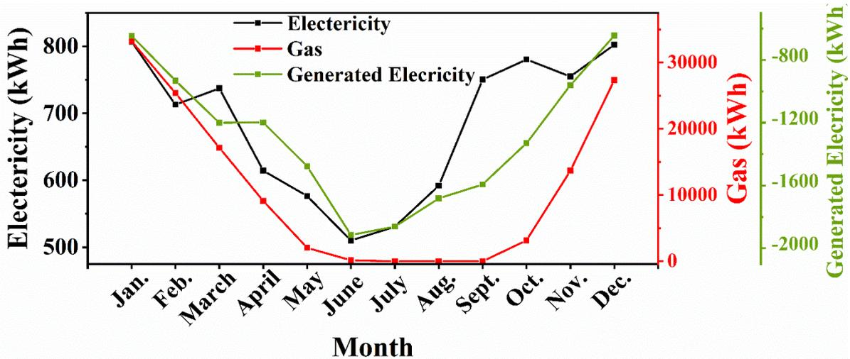
Figure 9: Fuel usage breakdown of retrofitted RB by PV panel; Electricity (black curve), gas (red curve), and generated power (green curve)
