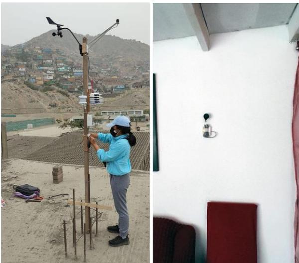
Figure 4. View of the outdoor weather station (left) and data logger inside a house (right).
