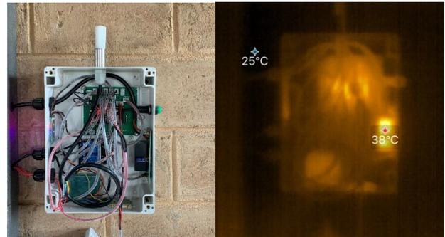
Figure 4: Thermal imaging of the IoT box
