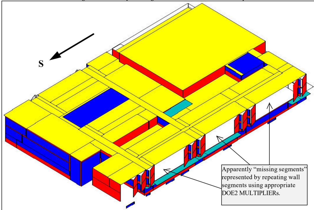
RUN 2. We removed the window positioning, allowing the window(s) to fall to the default lower left corner position within each containing wall surface.
