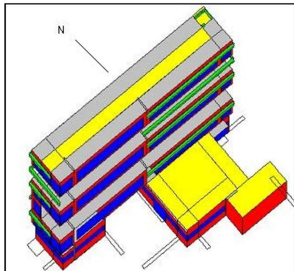
RUN 2 Beginning with the detailed model (run 1), we removed the interior surface positioning by modelling only the area and facing direction of interior surfaces. DOE2 uses a “split flux” method to model daylighting. It uses the reflectance and tilt of interior floors, ceilings and walls, but not the position of these surfaces (Winkleman, 1998).
