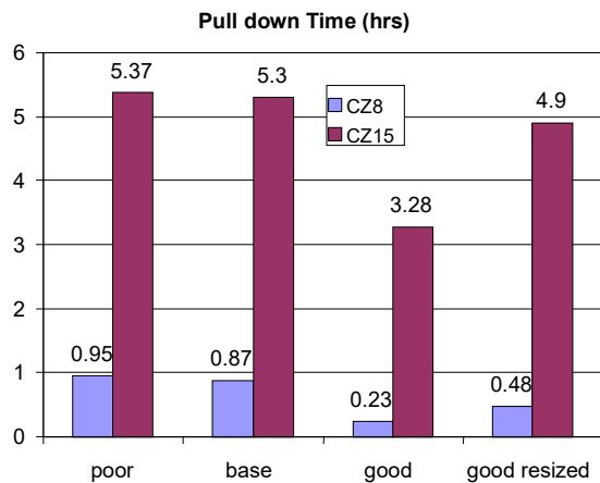
Figure 5. Climate and system dependence of the time required to cool a house (pull-down time)
