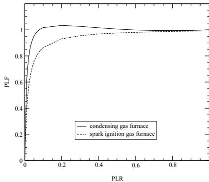
Figure 2: PLC for condensing & spark ignition furnaces.
