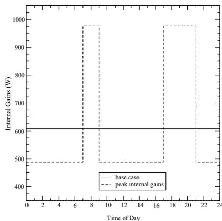
**Figure 8: Constant and peak internal gain profiles**
