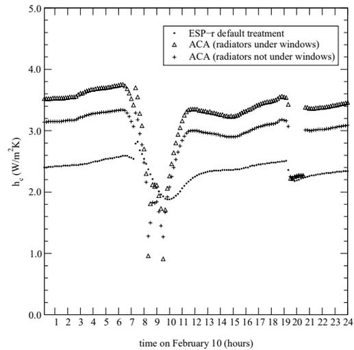
Figure 3: Impact of ACA on  $h_c$  calculations
