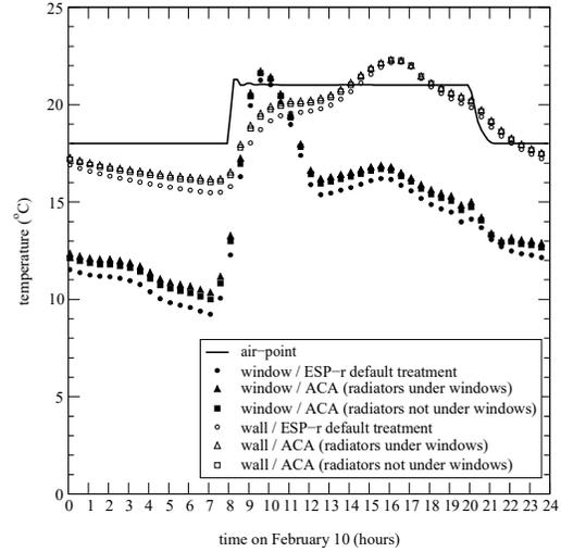
Figure 5: Impact of ACA on  $T_{air}$  and  $T_{surf}$
