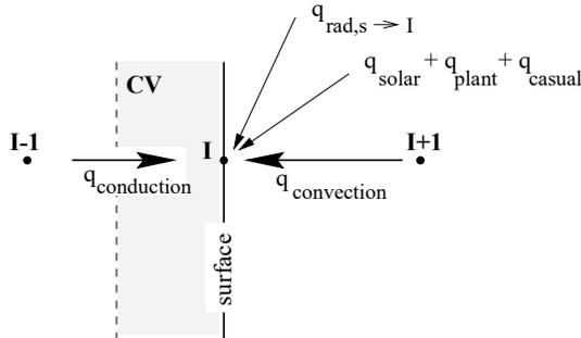
Figure 4: Heat balance at an internal surface
