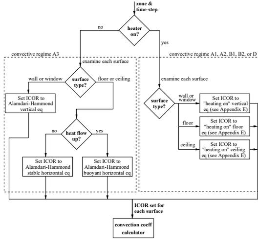
**Figure 2: ACA control law for terminal heating**
