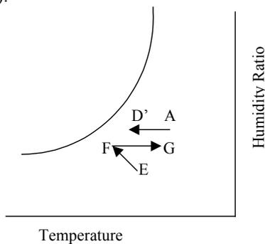
Figure 4: Psychrometric representation of indirect evaporative cooling system
