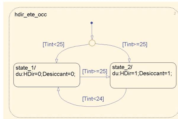
Figure 3: Graphical representation of the control of desiccant mode
