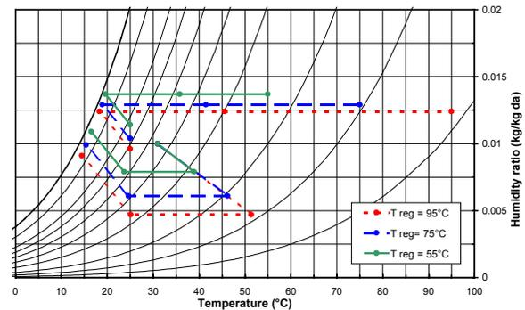
Figure 5: Psychrometric representation of an open desiccant cooling system for 3 regeneration temperatures
