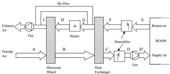
Figure 1: Schematic of a desiccant
