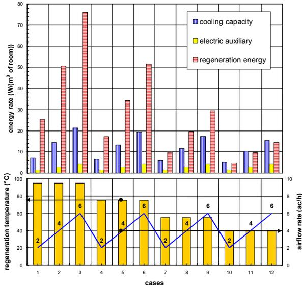
Figure 6: Impact of regeneration temperature and airflow rate on cooling capacity and energy rate for outdoor air conditions of 31°C and 35% and indoor air conditions of 25°C and 110g/h internal moisture gains
