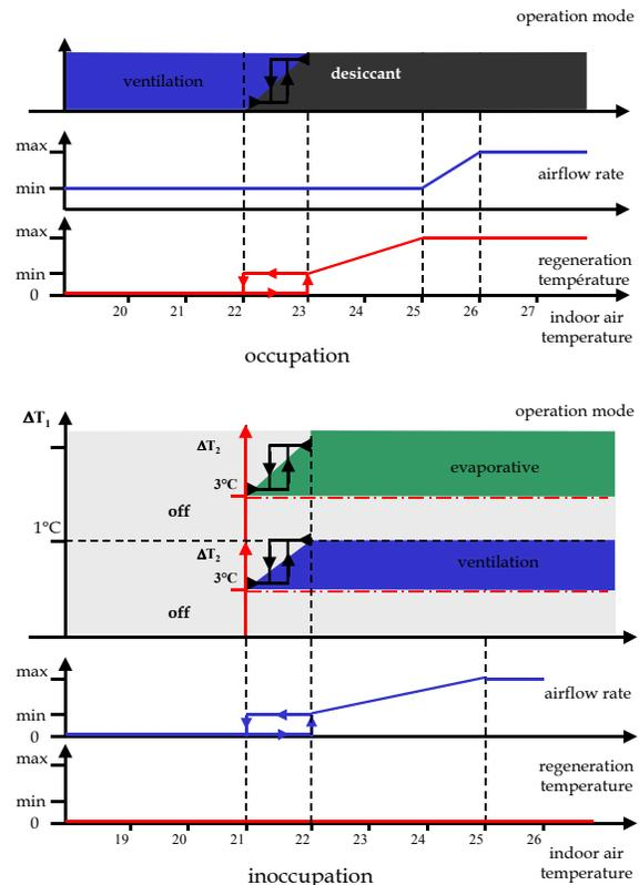
Figure 8: Control strategy diagram in case of free energy during day
