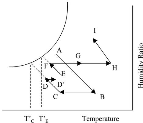
Figure 2: Psychrometric representation of desiccant cooling system
