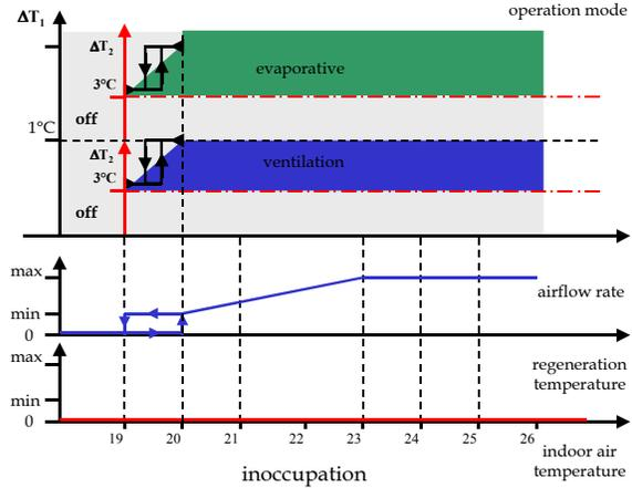
Figure 7: Control strategy diagram in case of purchased reactivation energy
