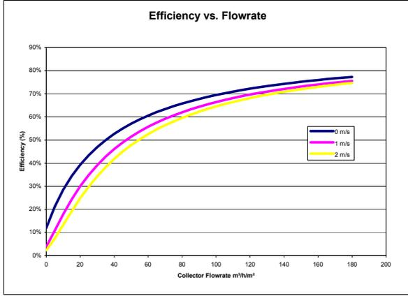
Figure 1 – Relationship Between Collector Efficiency and Collector Airflow at Various Wind Speeds
