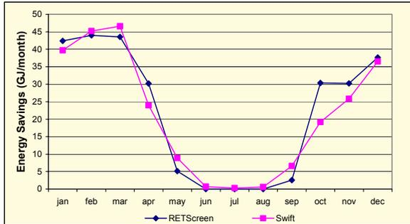
Figure 4 – RETScreen™ vs. SWift™ Total Savings (high-efficiency commercial system, Winnipeg)
