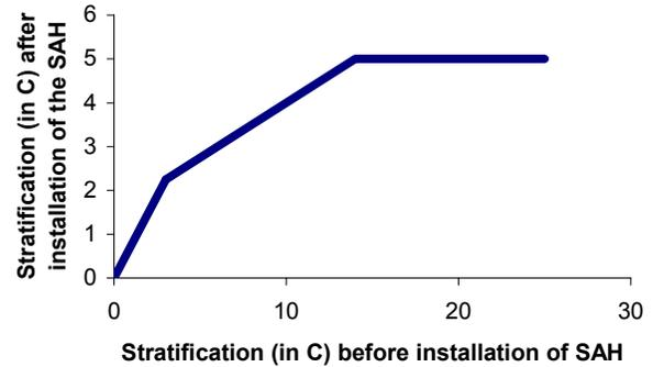
Figure 2 – Effect of SAH installation on building air stratification.
