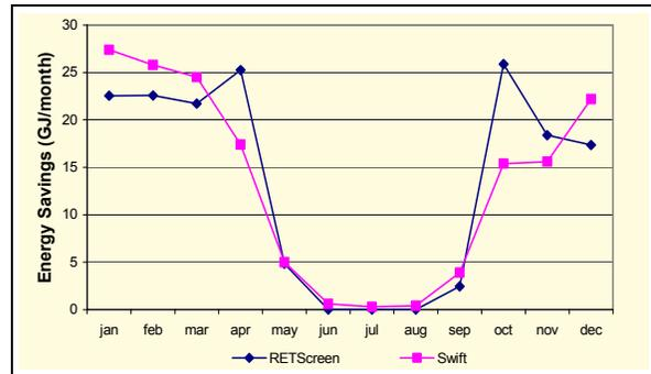
Figure 3 – RETScreen™ vs. SWift™ Total Savings (high temp-rise heating system for industrial building, Toronto).
