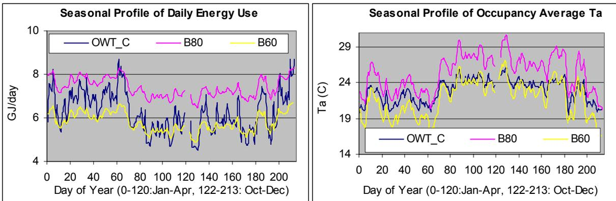
Figure 7 Comparison of annual performance between OWT and Type I boiler controller (Simulation in a system with uncontrolled terminals)
