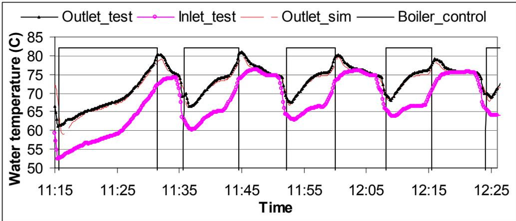
Figure 4 (b) Validation by test-rig data (floating Inlet temperature)
