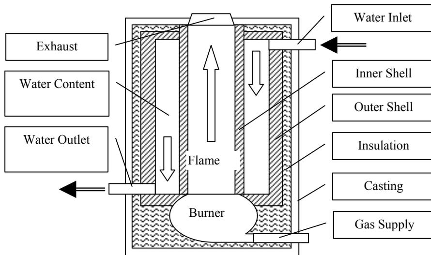
Figure 1 A simplified structure of gas or oil burned boilers
