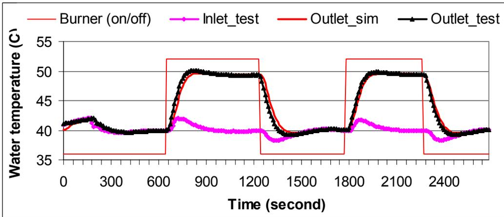
Figure 4 (a) Validation by test-rig data (constant Inlet temperature)
