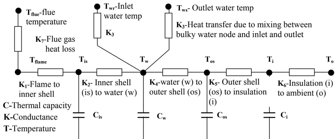
Figure 2 Electrical circuit model of a gas or oil burned boiler
