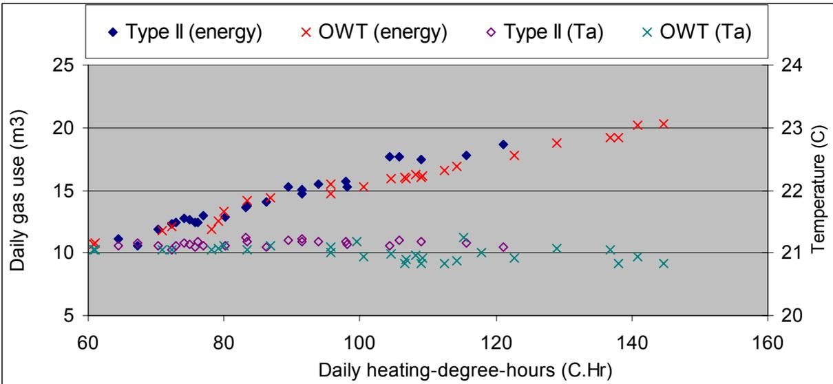
Figure 8 Comparison of performance between OWT and Type II boiler controller (Experiment in the ICITE testing facility)
