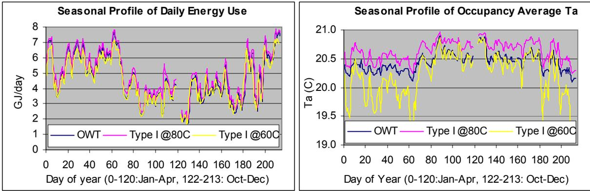
Figure 6 Comparison of annual performance between OWT and Type I boiler controller (Simulation in a system with well controlled terminals)
