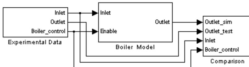
Figure 3 Validating the boiler model using experimental data
