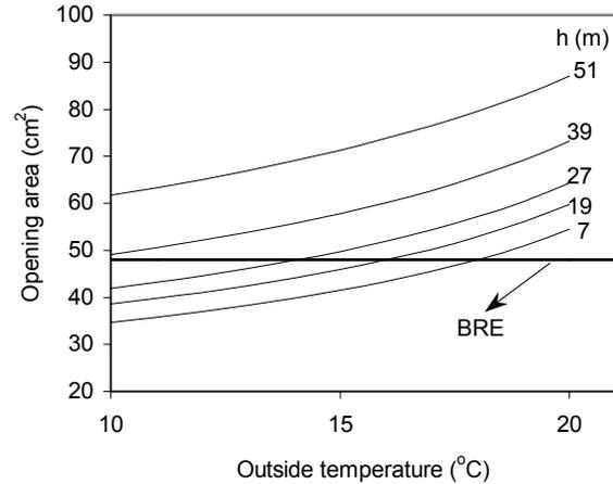
Figure 8. Opening area as a function of the outside temperature.
