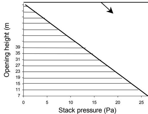
Figure 4. Stack pressure at the location of slot ventilators ( $T_o = 15^{\circ}\text{C}$ ).
