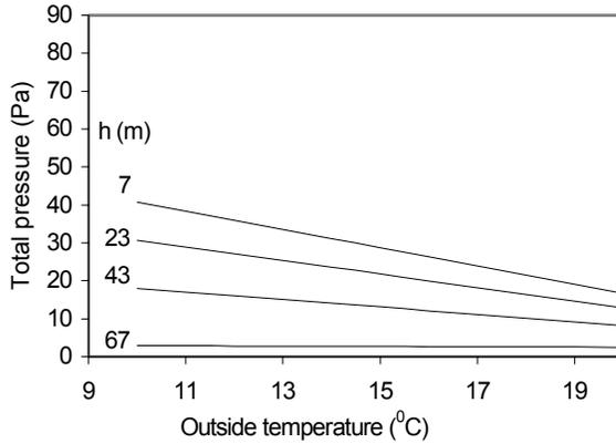
Figure 7. Effect of outside temperature on total pressure.
