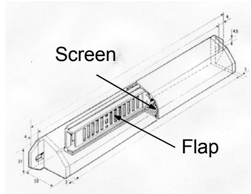
Figure 1(b). Pressure-controlled ventilator.
