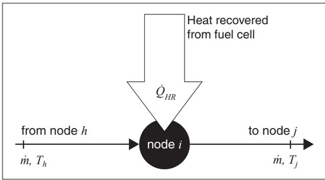
Figure 6: Arrangement of fuel cell component model in wet central heating plant.
