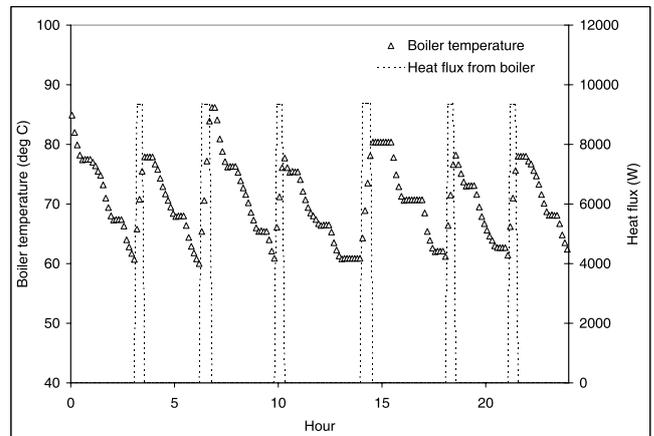
Figure 9: Boiler temperature and plant heat flux for wet heating plant without fuel cell.
