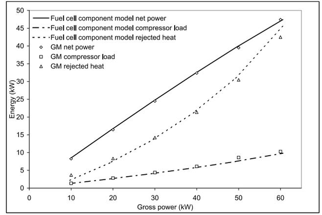
Figure 5: Comparison of fuel cell energy flow predictions, GM study and fuel cell component model
