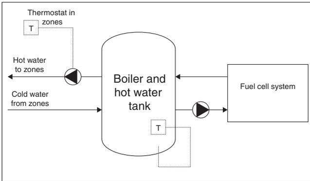
Figure 7: Arrangement of fuel cell component model in wet central heating plant.
