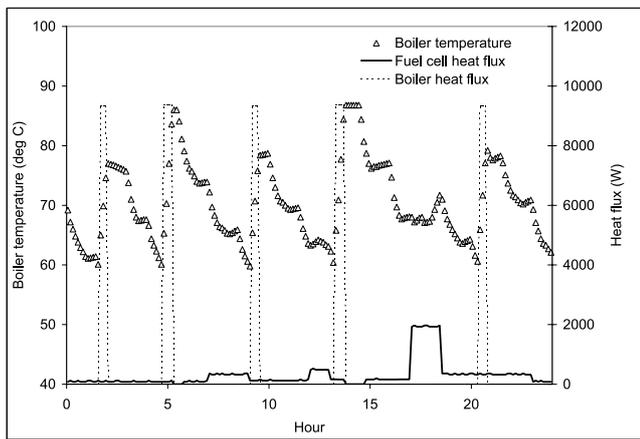
Figure 10: Boiler temperature and plant heat flux for a co-generation fuel cell system with variable electric output.
