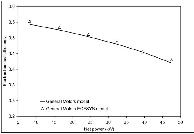
Figure 4: Comparison of fuel cell system efficiency estimates, GM study and fuel cell component model.
