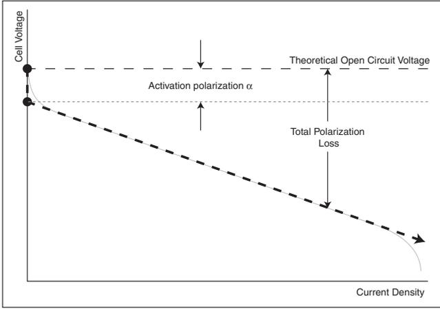
Figure 2: Simplified fuel cell polarization curve
