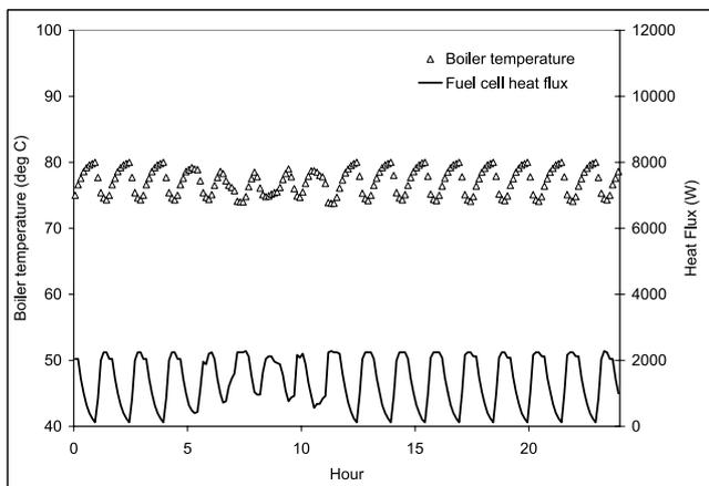
Figure 11: Boiler temperature and plant heat flux for a co-generation fuel cell system with constant 3kW electric output.
