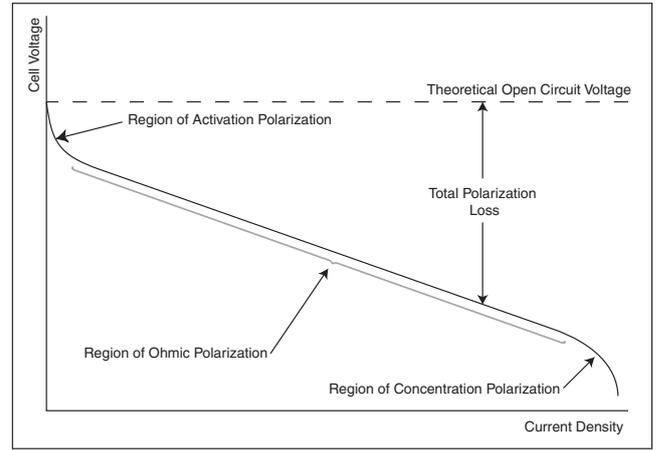
Figure 1: Typical fuel cell polarization curve
