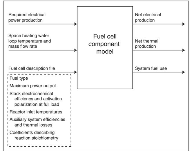
Figure 3: Inputs to and outputs from the fuel cell component model.
