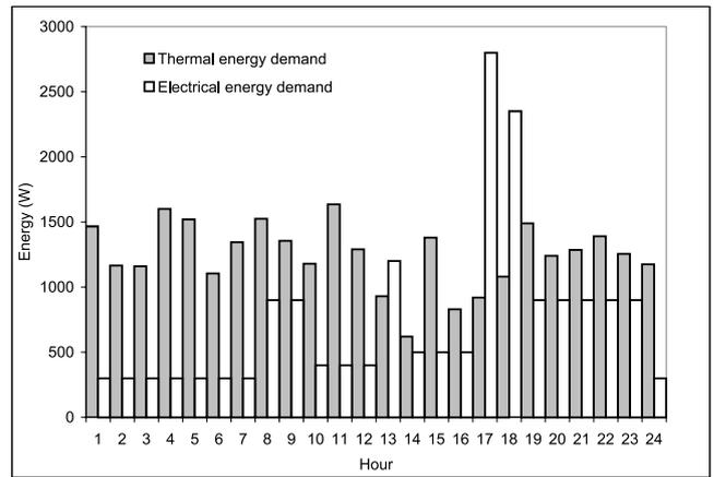
Figure 8: Load profile for a two-bedroom house in a temperate climate on an arbitrary winter day.
