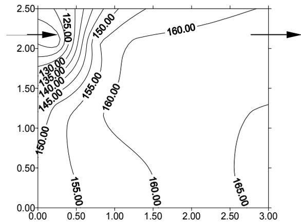
Figure 3 Nonane distribution at the middle section of the room (outlet at top, 1 hour)
