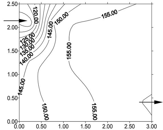
Figure 2 Nonane distribution at the middle section of the room (outlet at bottom, 1 hour)
