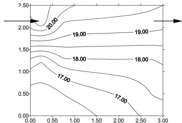
Figure 4 Temperature distribution in the middle section of the room (outlet at top)
