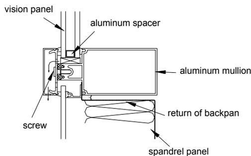
Figure 1a Joint section of a standard metal curtain wall
