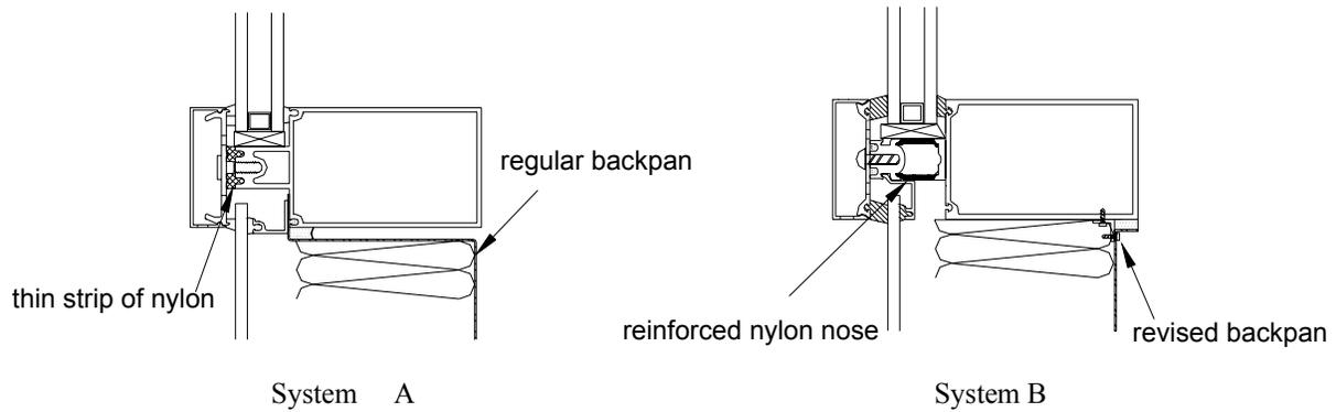
Figure 4. Curtain wall configurations simulated
