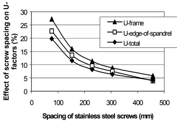
Figure 5. Impact of screw spacing on U-factor at the joint section for system A with standard IGU, regular back-pan
