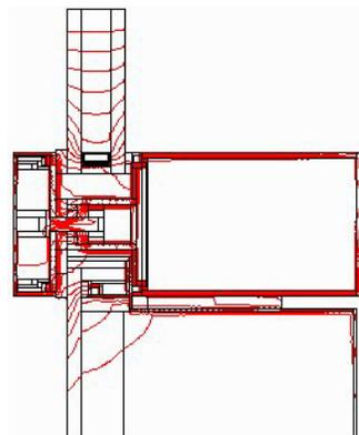
Figure 1b Heat flux across the joint section
