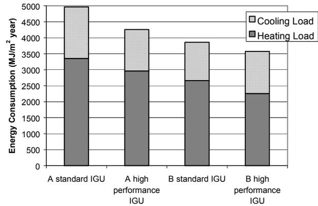
Figure 6 Comparison of energy consumption among four different curtain wall designs
