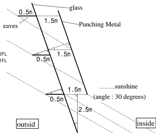
**Figure 3** Details of the building envelope of the gym
