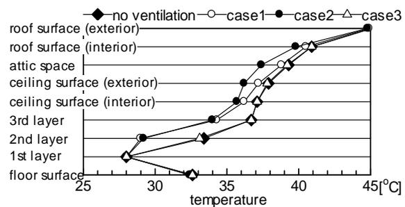
**Figure 10** Temperatures (Vertical Distribution)
