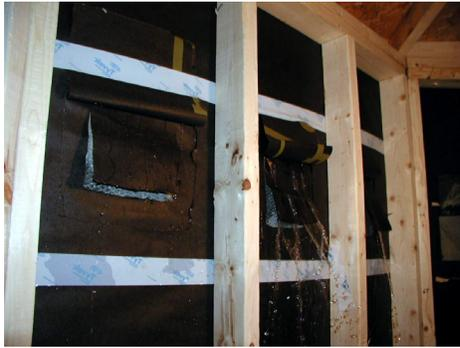
**Figure 2: Drainage capability of multilayers of building paper.**
