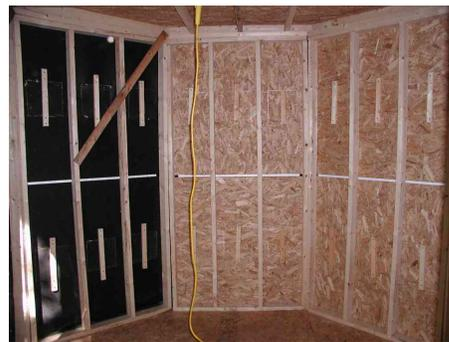
**Figure 1: JJAC water drainage/penetration set-up.**
