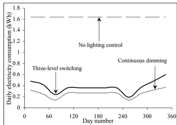
Fig. 12. Mean daily electricity consumption for lighting for the lighting control options (typical perimeter office on the SW façade).
