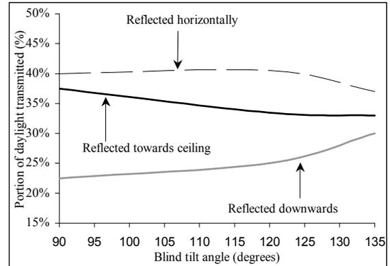
Fig. 4. Directional distribution of transmitted daylight through motorized venetian blinds, for different blind tilt angles.
