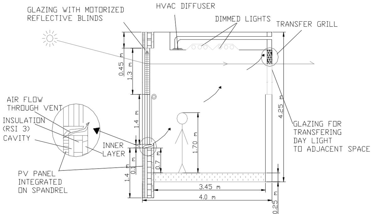
Fig. 1. The multifunctional façade with one daylighting - shading option for typical perimeter office.
