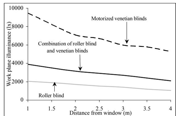
Fig. 5. Illuminance distribution in a typical office on the SW façade (July 15<sup>th</sup>, 1pm).
