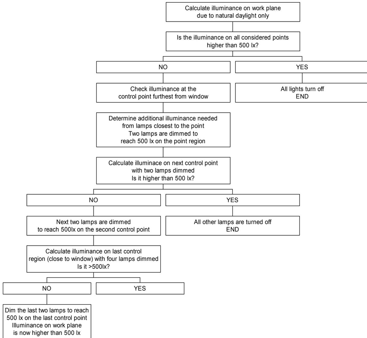
Fig. 11. The control algorithm for dimming
