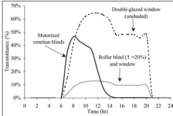
Fig. 3. Transmittance of shading devices (and window) as a function of time (July 15<sup>th</sup>).
