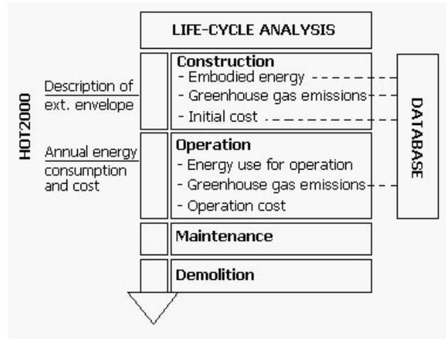
Figure 1. Flowchart of the EEE tool
