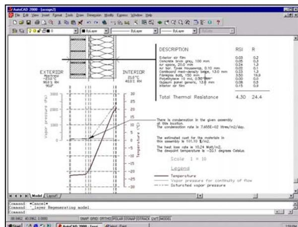
Fig1: Envelope section and the result in CONDENSE
