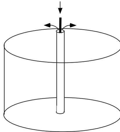
Figure 3: Borehole heat storage equipped with a C-pipe.
