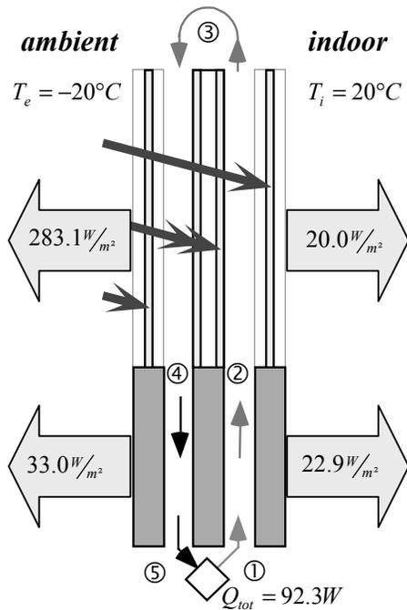
Figure 1: Results from the analytical steady state model of a double air gap wall and window construction with 4 panes.
