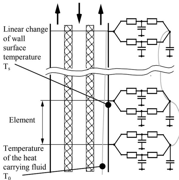
Figure 9 Possible Macro Element Method transformation model with half-5-node RC networks for a bore hole.
