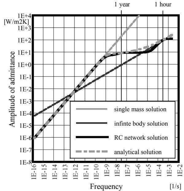
Figure 7: Amplitude of the admittance for a borehole wall in soil giving the analytical and the RC network solution and the asymptotes for single mass and an infinite external boundary.
