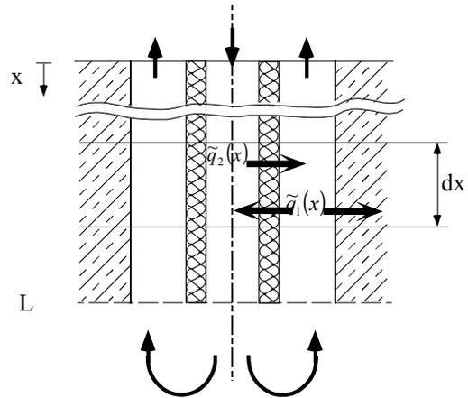
Figure 4: Borehole heat storage equipped with a C-pipe.
