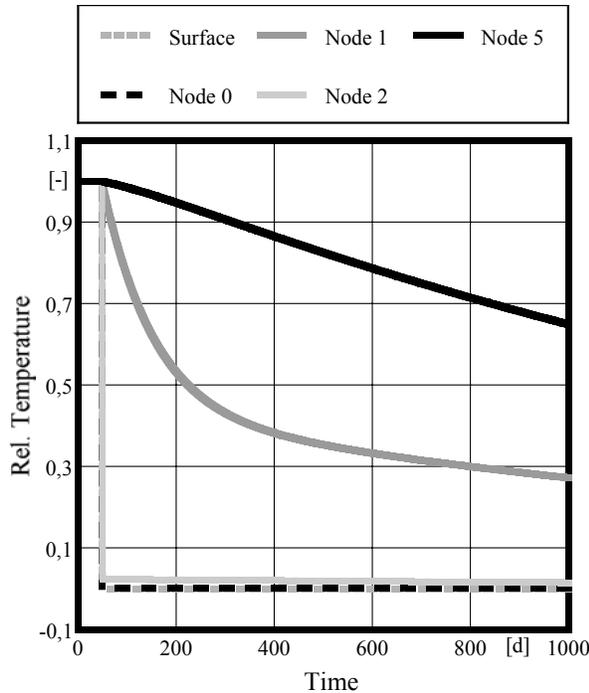
Figure 8: Calculation of the system response in time domain for the optimised RC network of a normalised relative temperature step of “1” at the surface.
