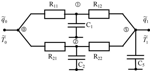
Figure 6: A half 5-node RC network modelling the thermal response at the surface 0 on a body with an adiabatic boundary in 1.
