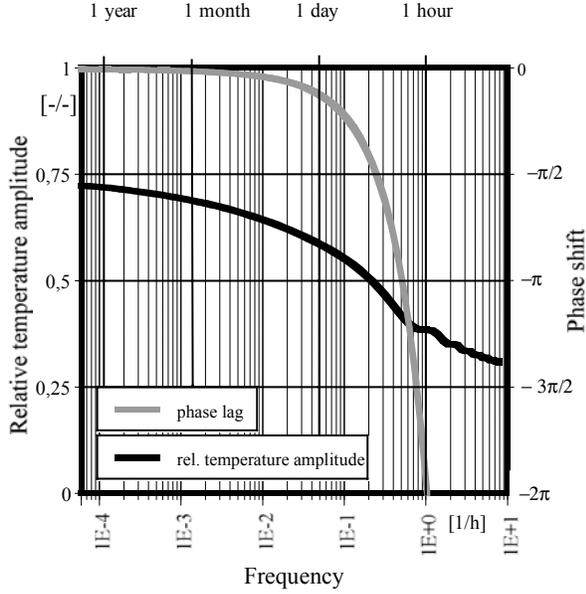
Figure 5: Temperature amplitude at the output of borehole vs. frequency of input temperature including heat exchange between the pipes  $\tilde{q}_2 \neq 0$ .
