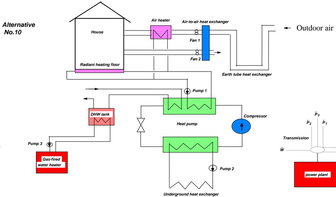
Figure 2 Configuration of the design alternative No.10
