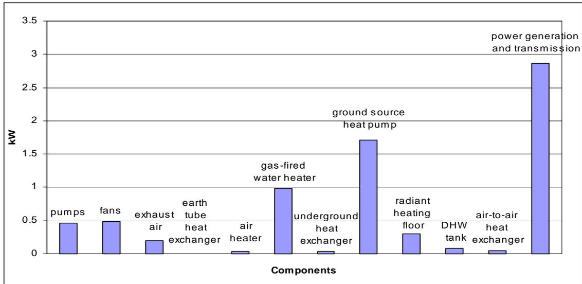
Figure 3 Exergy destruction for design alternative No. 10 at peak design condition (Total exergy destruction is 7.60 KW)
