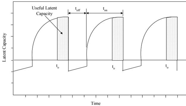
Figure 1. Variation of the latent capacity of the air-conditioner during quasi-steady operation showing effect of moisture evaporation during compressor off-time
