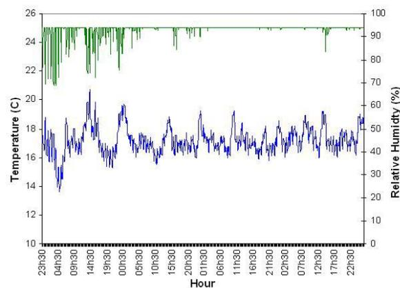
Figure 5. Main zone space temperature (left scale, upper plot) and relative humidity (right scale, lower plot) after the a/c re-evaporation model is activated.
