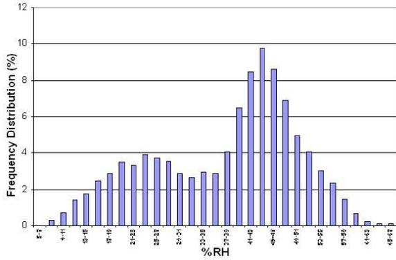
Figure 6. Main zone RH histogram after the a/c re-evaporation model is activated.
