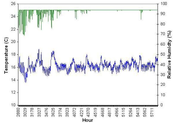
Figure 3. Main zone space temperature (left scale, upper plot) and relative humidity (right scale, lower plot) before the a/c re-evaporation model is activated.
