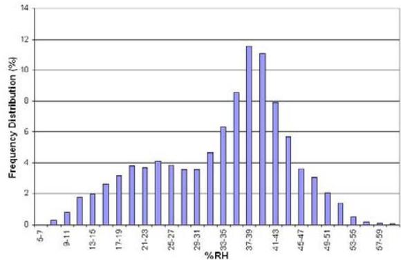
Figure 4. Main zone RH histogram before the a/c re-evaporation model is activated.
