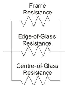
**Figure 2 Resistance Network of Window-Frame System. Note that inside and outside film, convective and radiation resistances are included in each component.**
