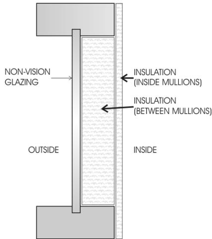
Figure 3 Schematic of Spandrel Panel
