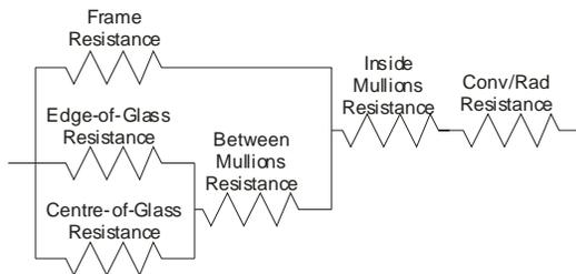
Figure 4 Resistance Network for Spandrel Panel. Note: Outside convective and radiation resistance is included in the frame, edge-of-glass and centre-of-glass values, however inside values have been removed.
