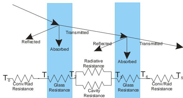
**Figure 1 Heat and Solar Radiation Path Modeled in Centre-of-Glass**
