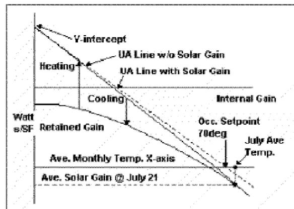
Figure 1. Method to Disaggregate Thermal Loads
