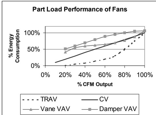
Figure 3. Example of Part Load Function
