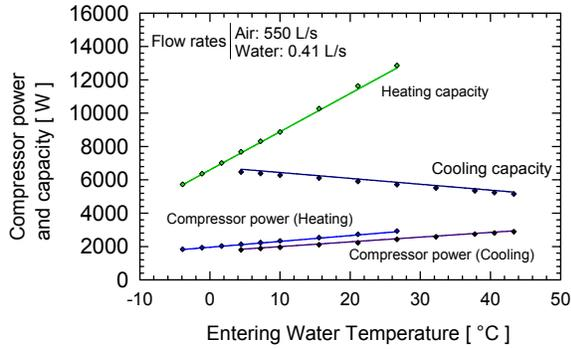
Figure 4: Heat pump performance data.
