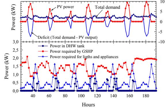
Figure 9: Power requirements and production for a typical winter week.
