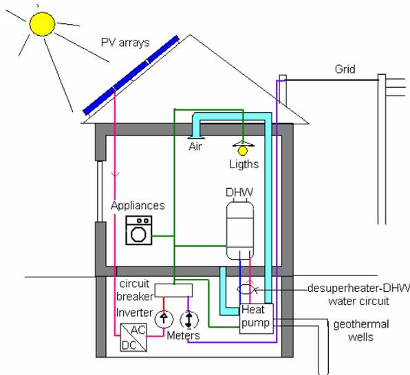
Figure 1: Schematic representation of the ZNEH studied.
