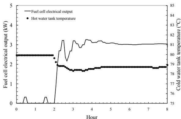
Figure 3: PID load following response to 2000 W step load on hot storage tank
