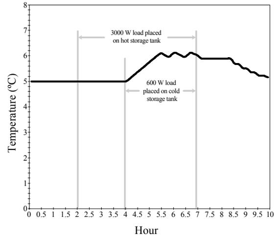
Figure 6: Cold storage tank temperature
