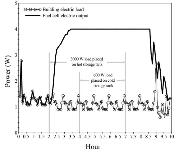
Figure 8: Building and HVAC electric loads, and fuel cell electrical production.
