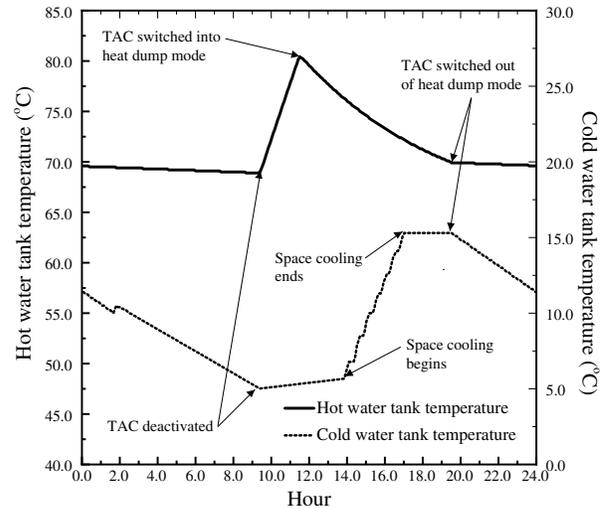
Figure 2: Hot and cold storage tank temperatures on an arbitrary summer day (June 1st).
