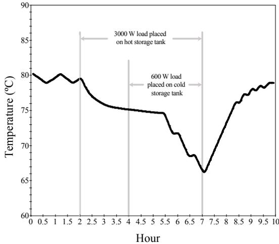
Figure 5: Hot storage tank temperature
