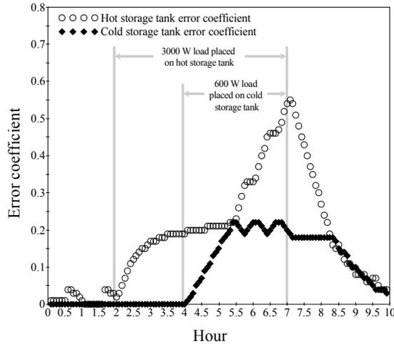
Figure 7: Hot and cold storage tank error coefficients.
