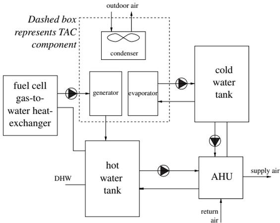
Figure 1: Schematic of residential CCHP plant.
