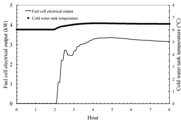
Figure 4: PID thermal load following response to 600 W step load on cold storage tank
