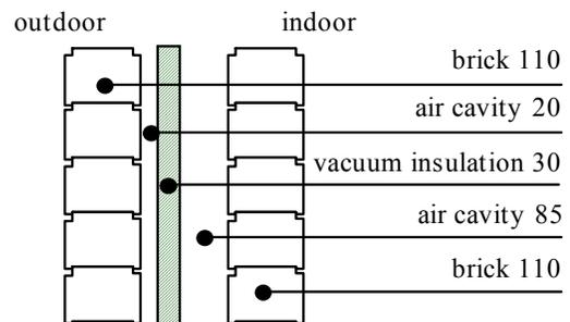
Fig.9 Exterior Wall Structure [unit: mm]
