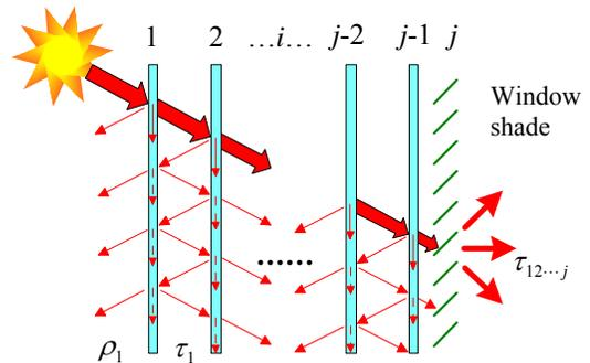
Fig.2 Multi-layer Window Model
