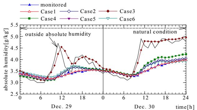
Fig.12 Comparison of Calculated Absolute Humidity with Different Conditions in Bedroom
