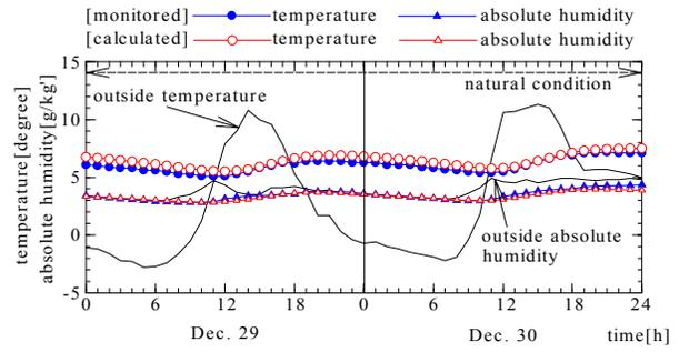
Fig.11 The Comparison of Monitored and Calculated Temperature and Absolute Humidity in the Cavity of the South Wall
