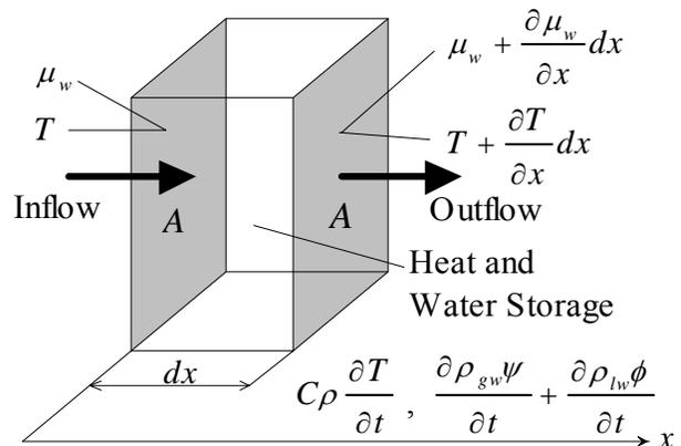
Fig.6 Conductive Heat and Moisture Transfer
