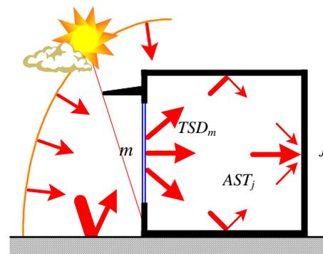
Fig.4 Multiplex Reflection of Transmitted Sky Diffuse Solar Radiation
