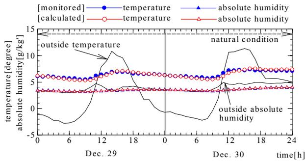
Fig.10 The Comparison of Monitored and Calculated Temperature and Absolute Humidity in the Master Bedroom
