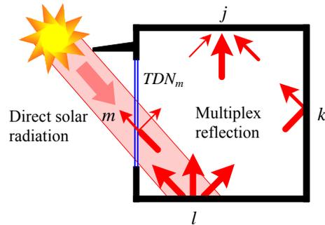
Fig.3 Multiplex Reflection of Transmitted Direct Solar Radiation
