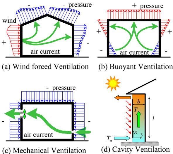
Fig.5 Mechanical or Natural Ventilation
