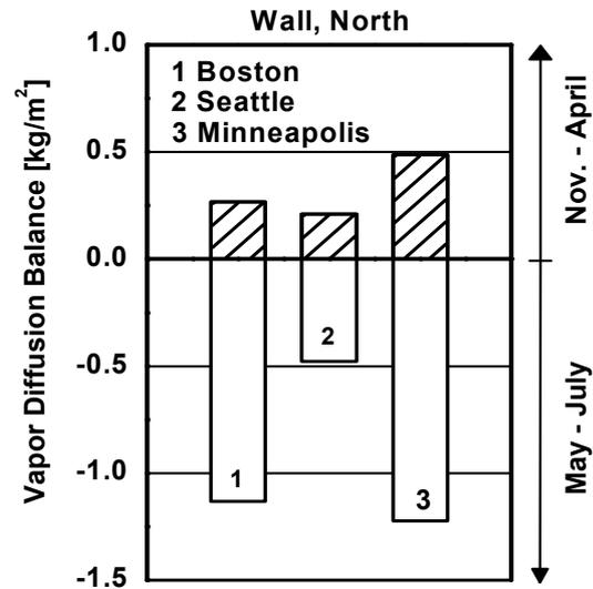
Fig. 7: Calculated vapor diffusion balance of the north facing wall with the variable-perm retarder (2 mil polyamide film) in Boston, Seattle and Minneapolis showing the maximum moisture content by condensation from November to April (hatched area) and the amount of moisture that dries out from May to July.
