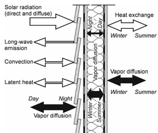
Fig. 1: Schematic representation of the hygrothermal effects and their alternating diurnal or annual directions in a wall construction.
