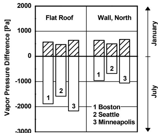
Fig. 5: Mean vapor pressure difference between the moist OSB sheathing of the building enclosure and the indoor air in January and July for 3 U.S. cities. Positive vapor pressure differences indicate condensation conditions and negative values quantify the drying potential of the building enclosure.
