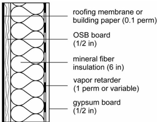
Fig. 4: Composition of the basic roof or wall assembly investigated by hygrothermal simulations
