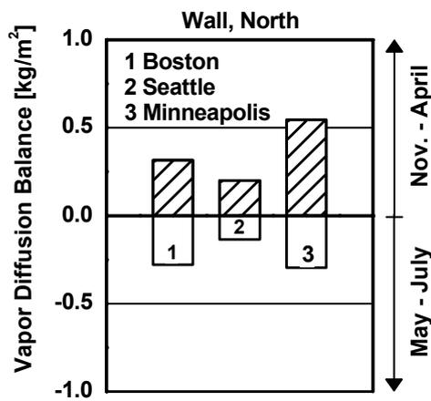
Fig. 6: Calculated vapor diffusion balance of the north facing wall with a one-perm retarder in Boston, Seattle and Minneapolis showing the maximum moisture content by condensation from November to April (hatched area) and the amount of moisture that dries out from May to July.
