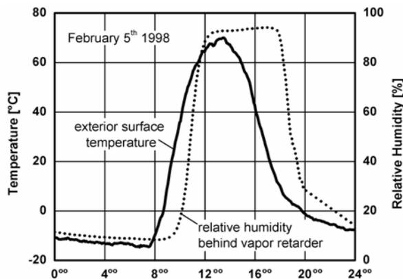
Fig. 2: Diurnal evolution of surface temperature and RH between the vapor retarder and the fiber glass insulation measured at a south facing cathedral ceiling during a sunny winter period in Germany.
