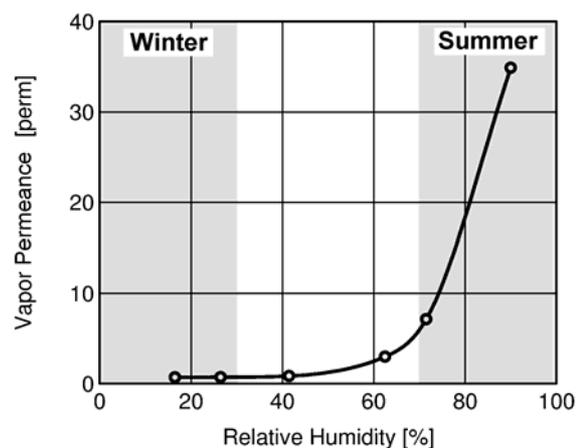
Fig. 3: Vapor permeance of a 2 mil polyamide film as a function of ambient RH
