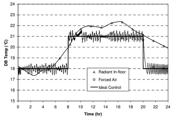
Figure 3: Forced Air & Radiant Temperature Profile Comparison for Mainfloor: DBT Sensed (Ottawa, Jan 9<sup>th</sup>)
