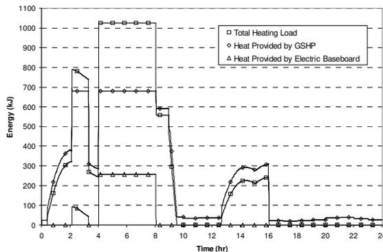
Figure 2: Primary & Secondary HVAC End-Use Energy Consumption (Ottawa, Jan 9<sup>th</sup>)
