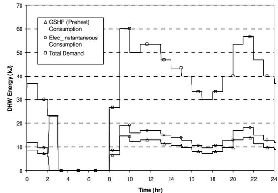
Figure 5: DHW Preheat End-use Energy Consumption for Jan 9<sup>th</sup>
