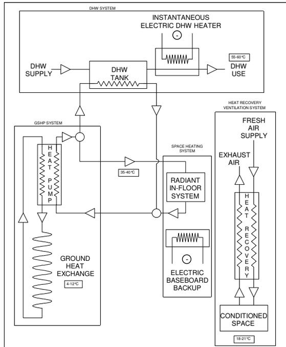
Figure 1: Schematic of Proposed Hybrid HVAC System
