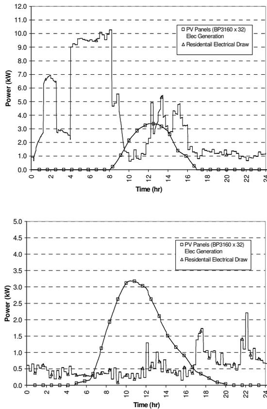
Figure 6: PV Electricity Generation vs. Electrical Draw for Day in Winter (top) and Summer (bottom)
