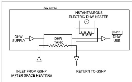
Figure 4: Schematic of DHW System Model
