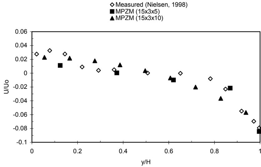
Figure 6 Comparison of the MPLM predictions with measured data at  $x = 1.0\text{m}$  for ceiling inlet.
