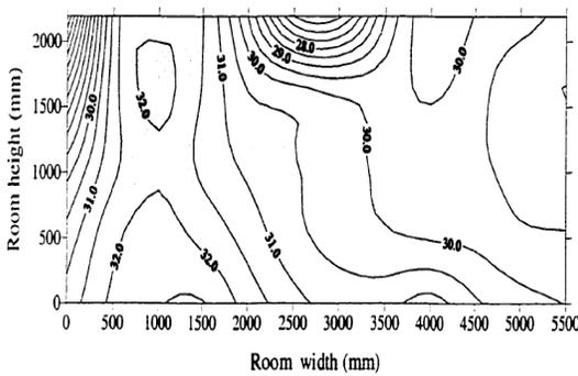
Figure 9 Measure temperature distribution (Zhao, 2000).
