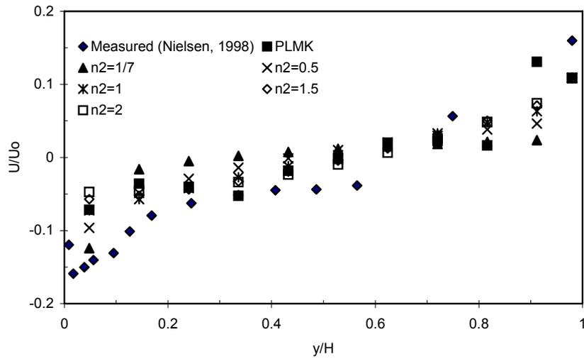
Figure 4 Comparison of the MPLM predictions for different values of  $n_1$  and  $n_2$  with measured data at  $x = 3m$  for wall inlet.
