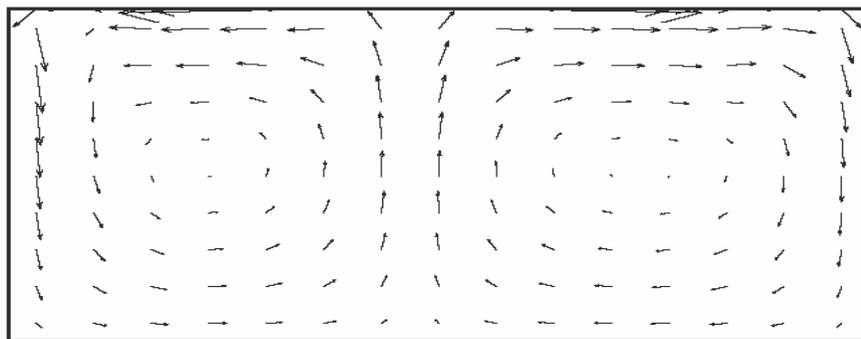
Figure 5 Airflow pattern predicted by the MPLM using 15x3x10 cells for ceiling inlet.
