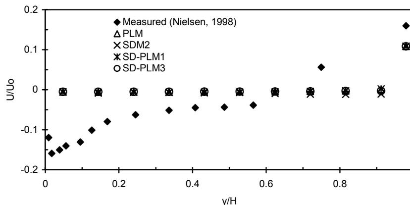
Figure 1 Comparison of the zonal models predictions with experimental at  $x = 3\text{ m}$  for wall inlet.
