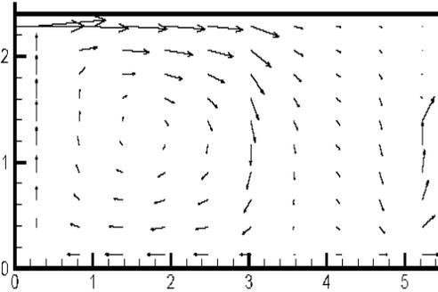
Figure 8 The MPLM airflow pattern prediction for non-isothermal room.
