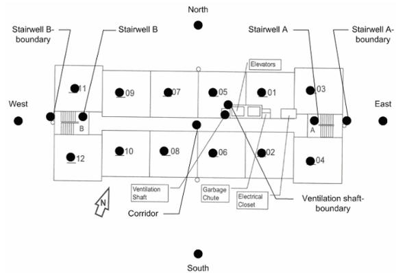
Figure 3. The airflow network nodes.
