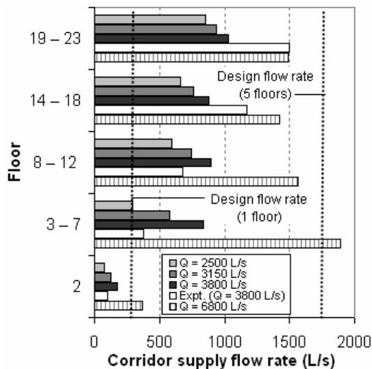
Figure 5. Corridor supply flow rate for different floors (February 12, 2001) with the supply fan ON.
