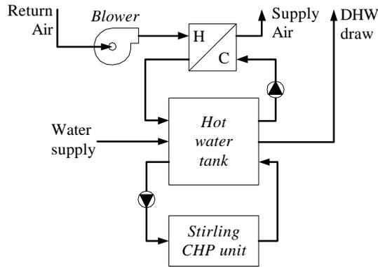
Figure 3: Arrangement of Stirling CHP unit in CCHT mechanical plant.
