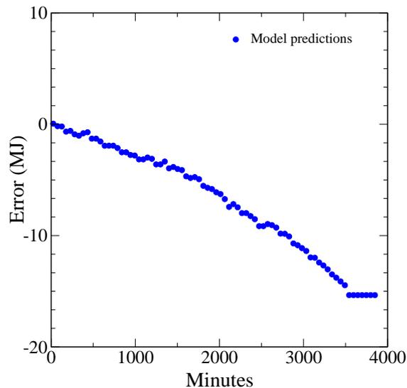
Figure 6: Cumulative difference between CCHT test data heat recovery measurements and model predictions (data-points represent every 50th measurement)
