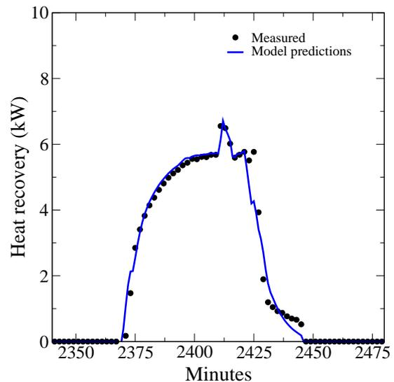
Figure 5: Comparison of measured rate of heat recovery and predicted values for CCHT calibration data: 2350–2475 minutes
