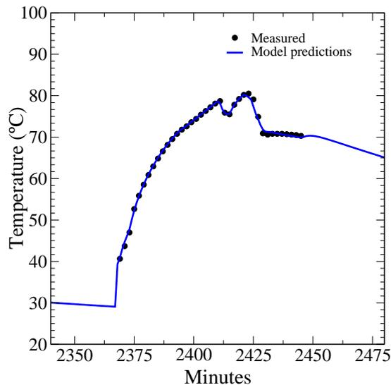
Figure 4: Comparison of measured outlet temperature and predicted values for CCHT calibration data: 2350–2475 minutes
