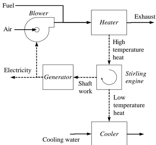
Figure 1: Mass flows (solid lines) and energy flows (dashed lines) in simple, combustion-based Stirling CHP system
