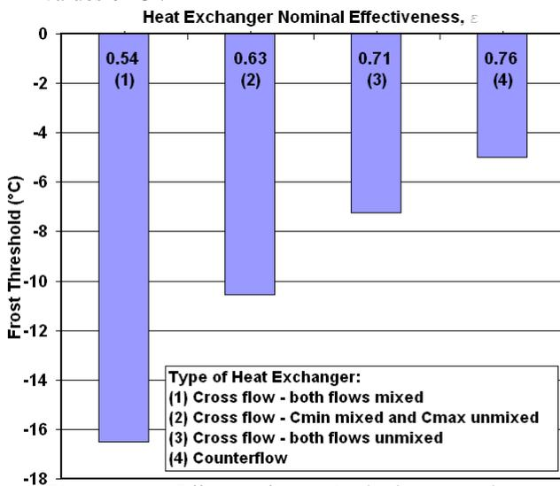
Figure 4. Effect of nominal heat exchanger effectiveness,  $\epsilon$ , on frost threshold temperature,  $T_{f,th}$
