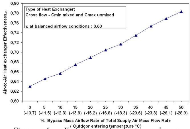
Figure 5. Variation of heat exchanger effectiveness,  $\epsilon$ , with bypass mass airflow rate percentage and outdoor air temperature
