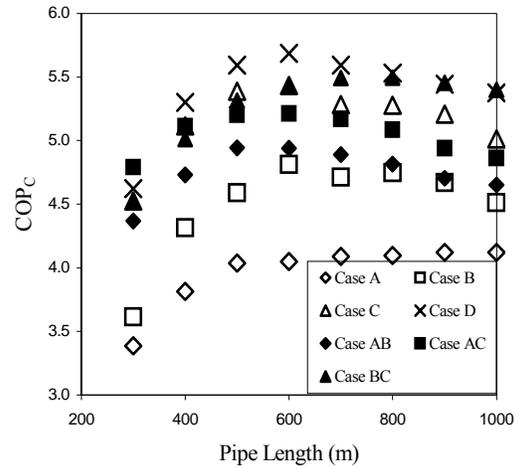
Figure 3. Variation of seasonal cooling COP of a GCHP system with pipe length for a GHE at various depths.
