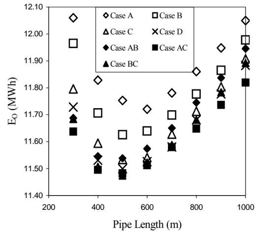
Figure 5. Variation of total energy consumption of GCHP system with pipe length for a GHE at various depths.
