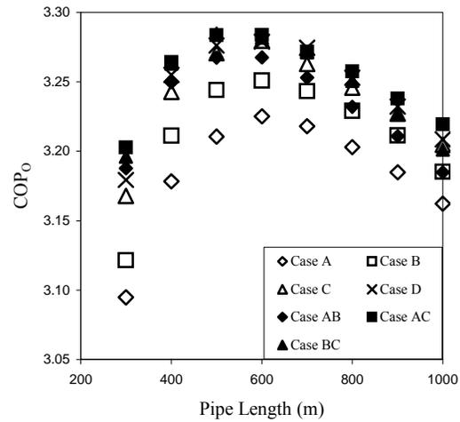
Figure 4. Variation of overall COP of GCHP system with pipe length for a GHE at various depths.
