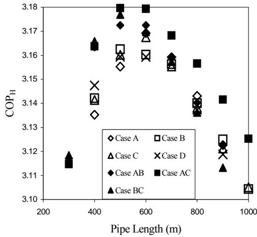
Figure 2. Variation of seasonal heating COP of the GCHP system with pipe length for a GHE at various depths.
