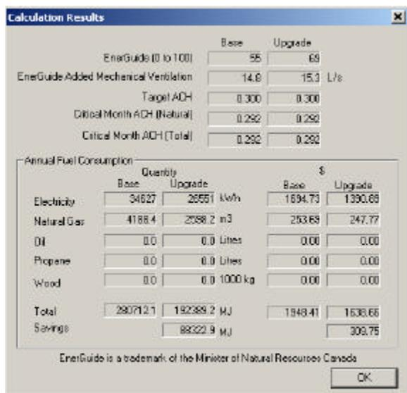
**Figure 4.** Typical screen display of energy analysis results.
